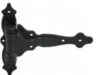
This Mini-Multi TCAMA1 hinge is designed to fit gate gaps up to  $38 \text{mm} \ (1\frac{1}{2})$  with square corner posts and gates. Horizontal and vertical adjustment using slots.
