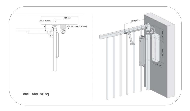
The two earlier pages have shown how you can install a Verticlose with the two common hinge arrangements, in-line and offset. There is another arrangement which is to mount to a wall or block work.
